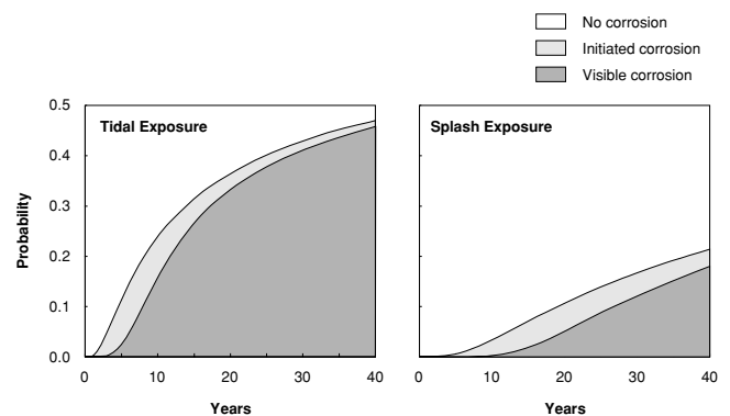
Fig. 4. Differences in initial probabilities of the different condition states for the same structure assuming two different exposure classes. The left figure corresponds to Figure 3.
