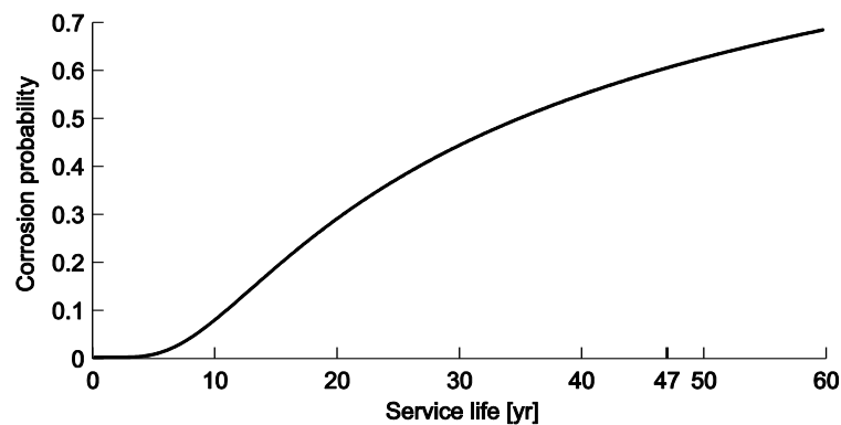
Figure 5: Prior corrosion probability of the reinforcement calculated with MCS.
